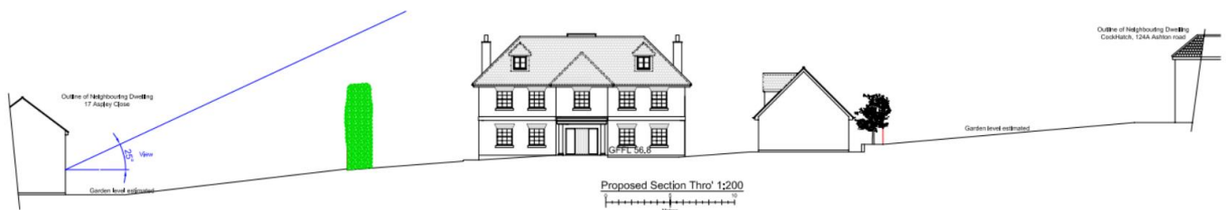
Site section north - south across the site showing the proposal's relationship with the house to the north and the property to the south.
